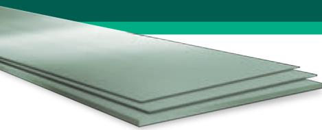
**QUARD 450** is a martensitic abrasion resistant steels, with an average hardness of 450 HBW. The steel offers very high resistance to abrasive wear and impact granting a longer service life. The combination of very good cold forming properties and excellent weldability makes **QUARD 450** an optimal choice for most wear applications.
