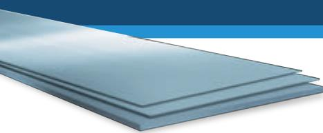
**QUEND 700** is extra high strength structural steel produced as quenched and tempered with a minimum yield strength of 700 MPa. **QUEND 700** complies with the requirements corresponding to the S690QL given in the EN 10025-6 standard, where a minimum impact toughness of 27 J is guaranteed at -40°C.
